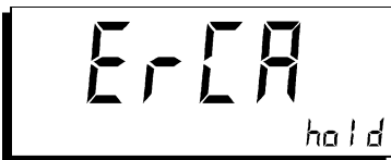
Figure 4-21 The data set stored for the plugged-in probe has a checksum error and cannot be used.
