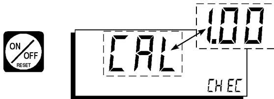
Figure 4-4 The self-test runs immediately after switch-on
