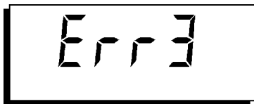
Figure 4-18 An error was detected during the self-test.
