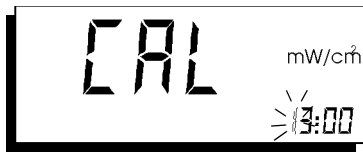
Figure 4-13 CAL display. The calibration factor setting is displayed in the lower right corner. The digit which can be altered flashes in the display.
