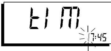
Figure 4-34 Entering the time of day; the digit being edited flashes
