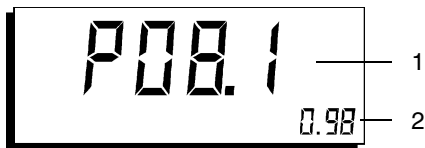
Figure 3-6 EMR-200/-300 display after probe is plugged in 1 Probe type and version 2 Relative sensitivity rounded to two places
