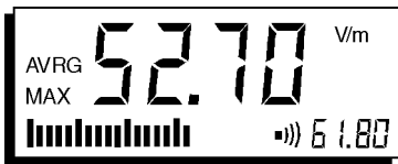
Figure 4-5 The device is ready for use when the measured value and other display elements are visible
