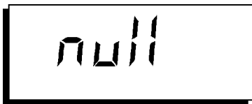
Figure 4-17 Display during automatic zeroing
